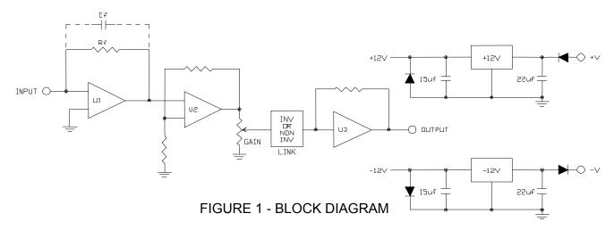
The components used in the different models are selected for voltage and current noise to provide an optimum combination of noise, gain and bandwidth.
