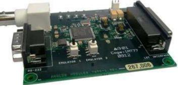
Pass-thru mode that allows RS232 host system (such as standard PC) to communicate with an AMI LRF Receiver Range-Processor connected to the LVTTL interface. The 7555 Interface Test Board provides buffering and baud rate translation.
